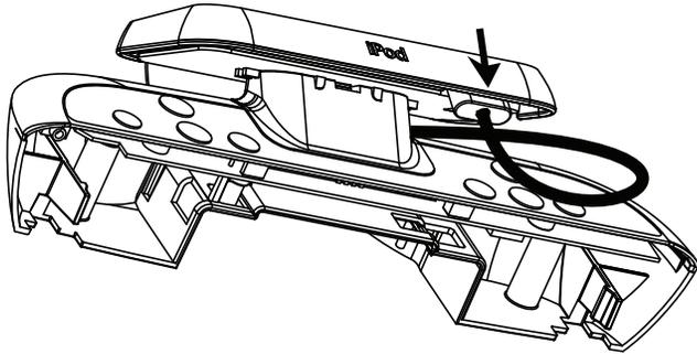
2. Use a small flathead screwdriver to depress the tab on the tray mount and slide the tray off the tray mount.
