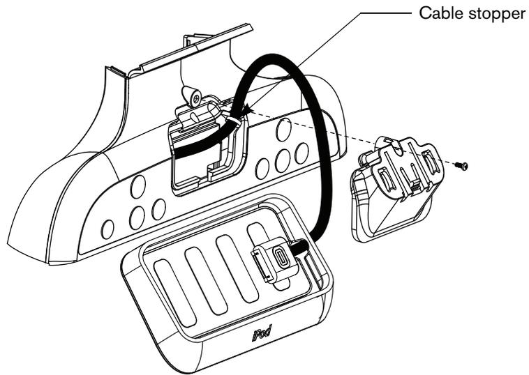
7. Slide the tray into place. You should hear an audible click when it snaps securely into place.
