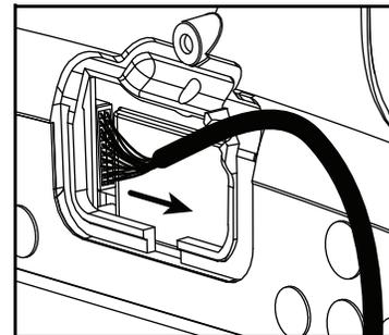
5. Slide the white connector end of the new cable through the tray and attach it to the receptacle in the PEP. You should hear an audible click from the connector when it snaps securely into place.
