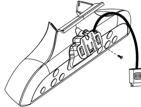
4. Pull firmly on the cable end attached to the PEP to remove it.
