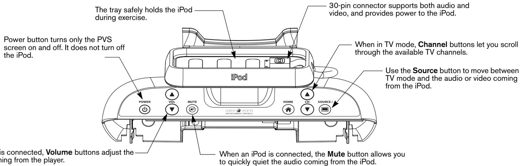
**Figure 1: Overview of the integrated PEP controller**
